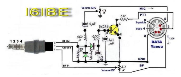
As shown in the image above, the circuit uses the BC237 to key the transceiver using an open collector configuration; Audio in and out is adjusted to suit the software and mode using R2 and R5. With a low component count (only12), this is the ideal weekend project for the aspiring Digital Mode Operator. Thanks to Eddie using it out in the field while taking part in RaDAR is now a definite must for all.
